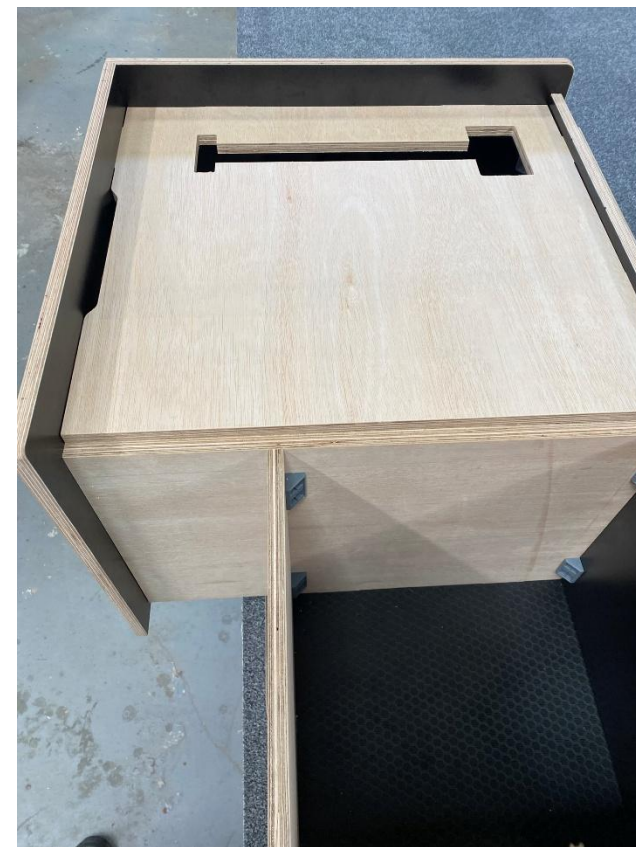
Fit A17 seat base then A2, LWB A2 differs to picture
