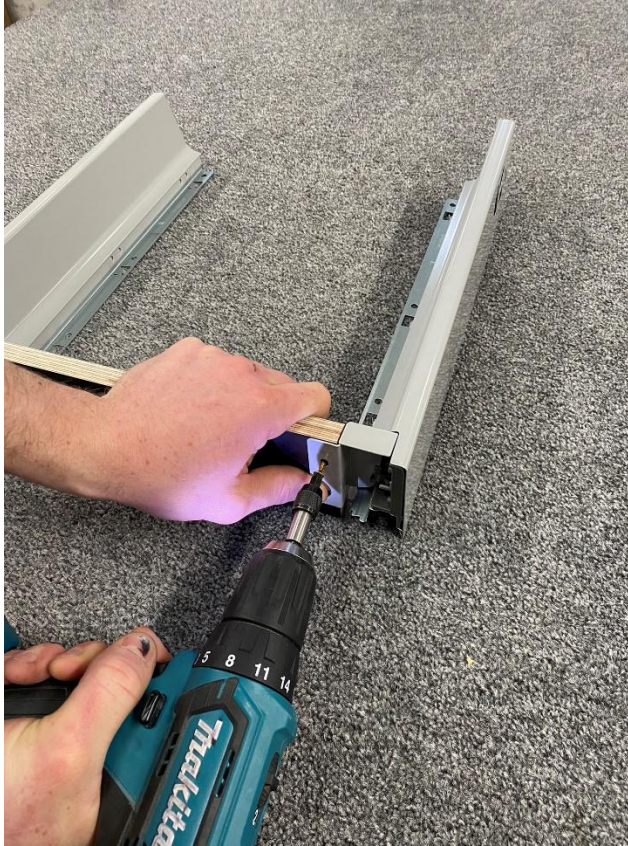
Fit the drawer rear using 15mm screws. Fit 9722 C11 drawer rear in kitchen pod when fitting the 9722 grill
