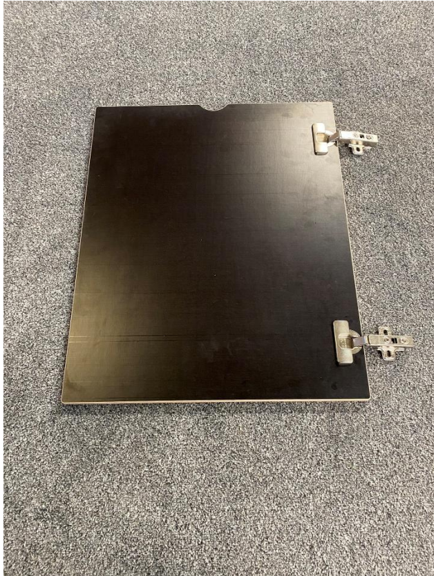
Fit overlay hinges to C7
