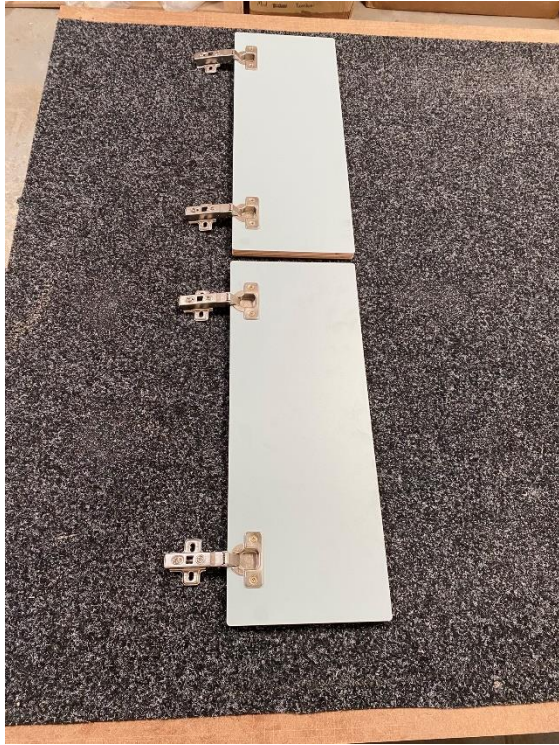
Fit the hinges into the doors
