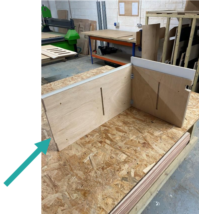
Screw 10 to 16 using 25mm screws, ensure orientation is correct with both rebates flush together
