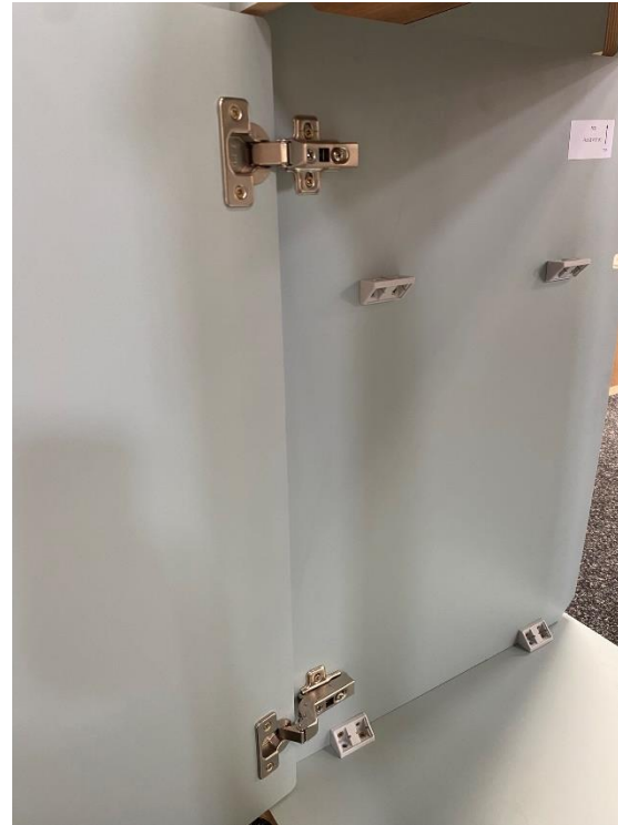
Hang the fridge door
