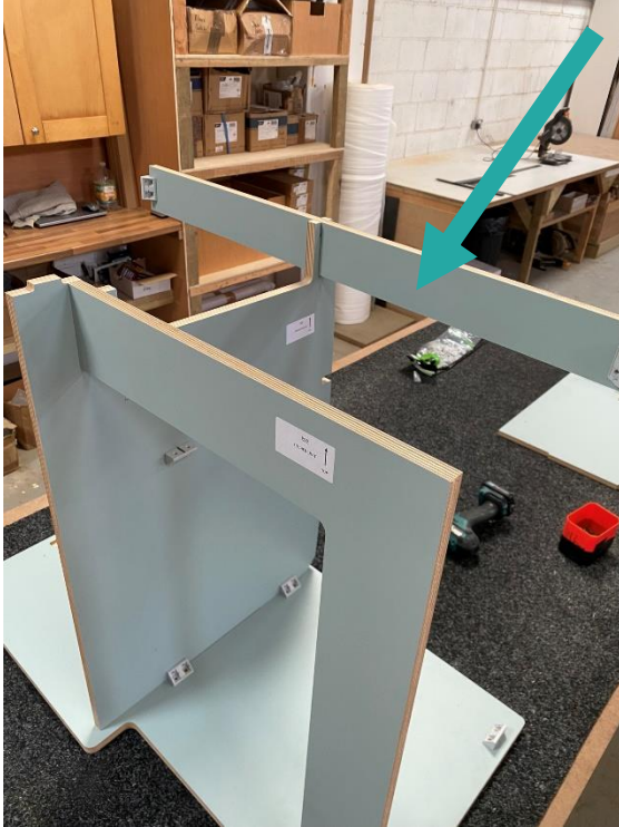
Attach the rear support over the fridge pod (R) and into the right end panel
