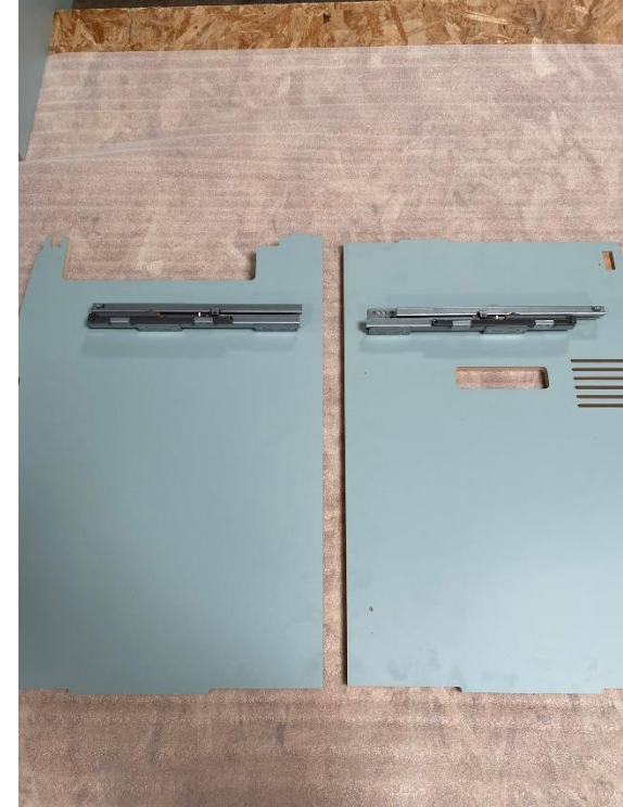
Fit the drawer runners to the fridge pods, no blocks are required this time, ensure orientated correct
