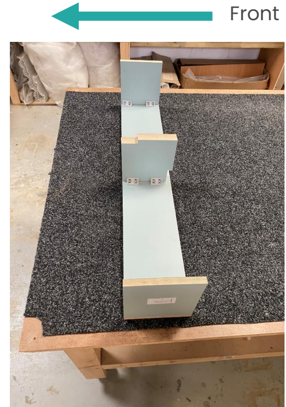
Fit the end panels
