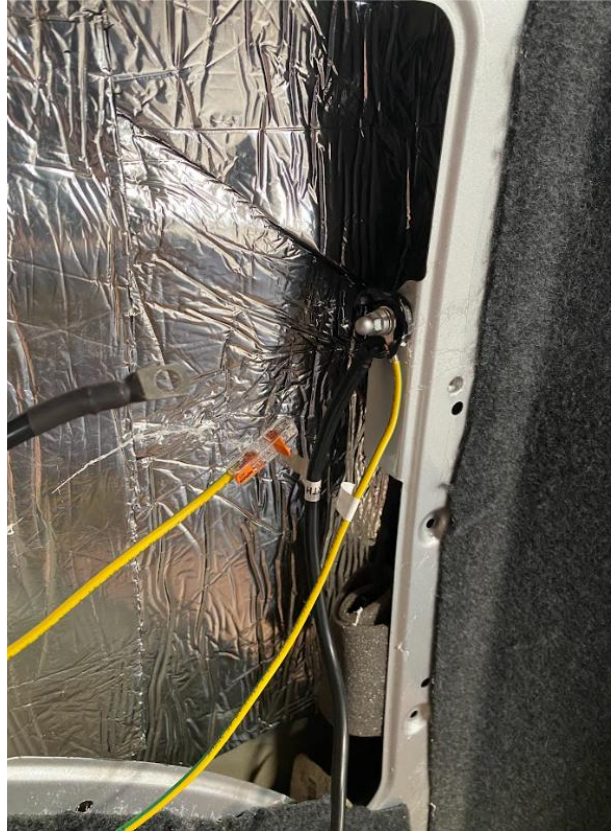
Fit the earth cables
