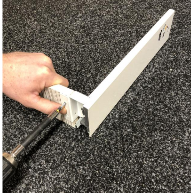
Fit the drawer rear using 15mm screws
