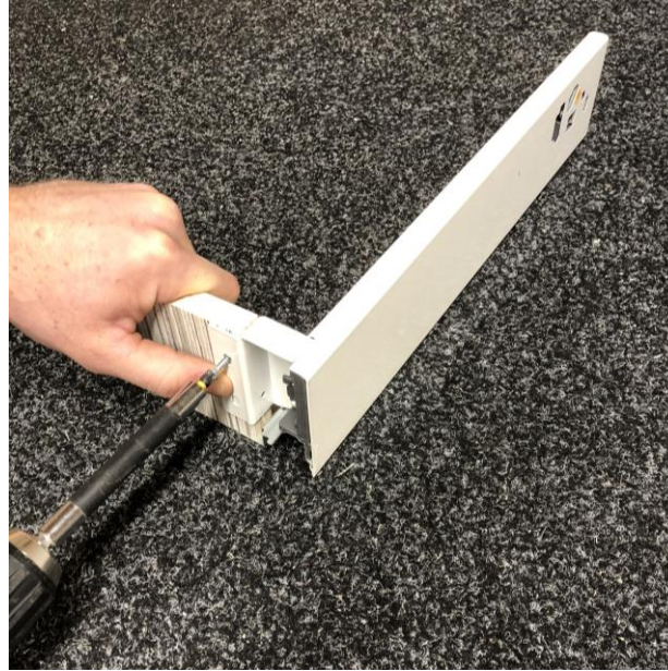
Fit the drawer rear using 15mm screws
