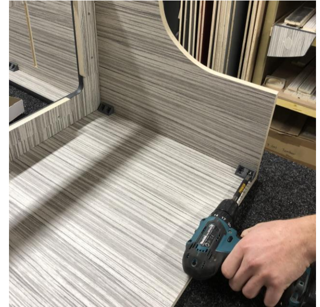
Fit the wardrobe upright (L) first, start from the base working up to the top using the blocks and pilot holes
