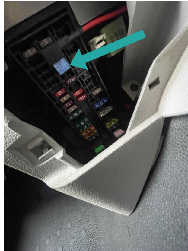
Insert the 15amp fuse into the piggyback and fit in the same location
