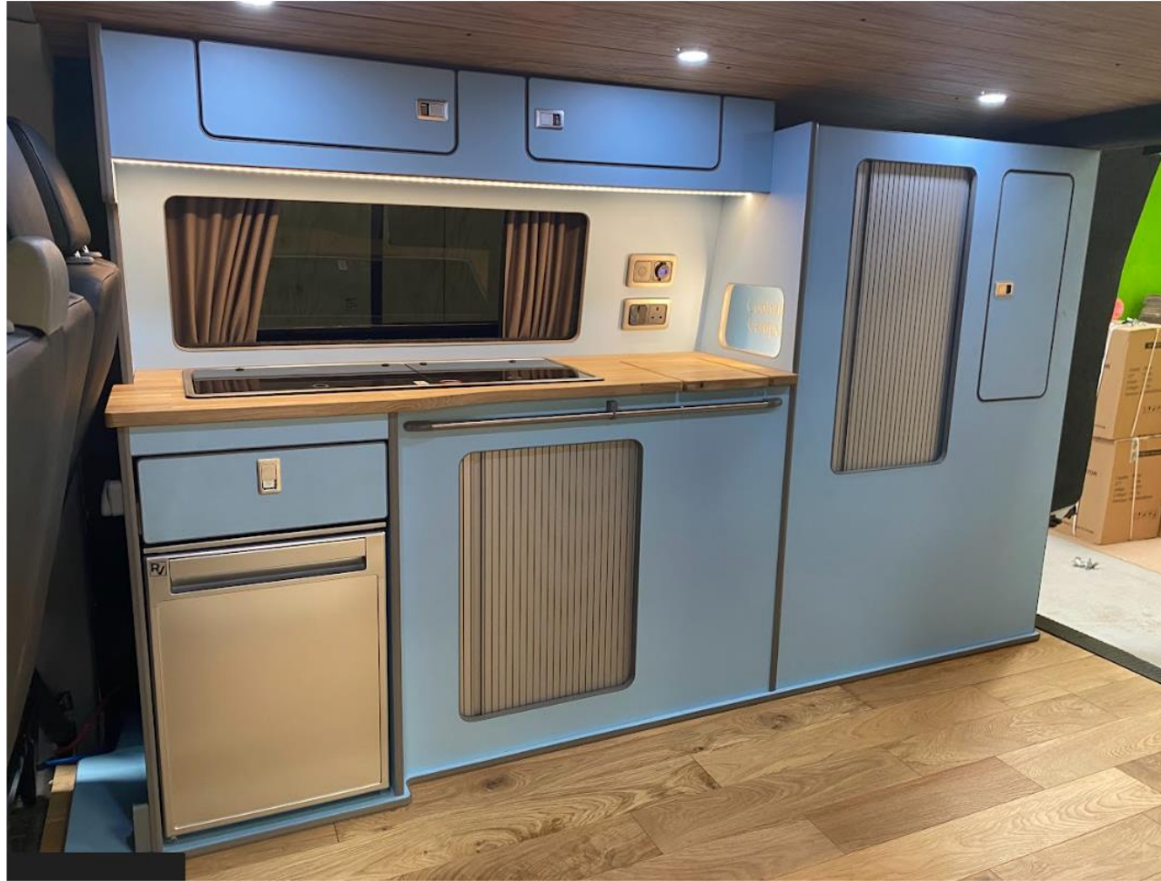
Offer the units into position but do not fit into place
