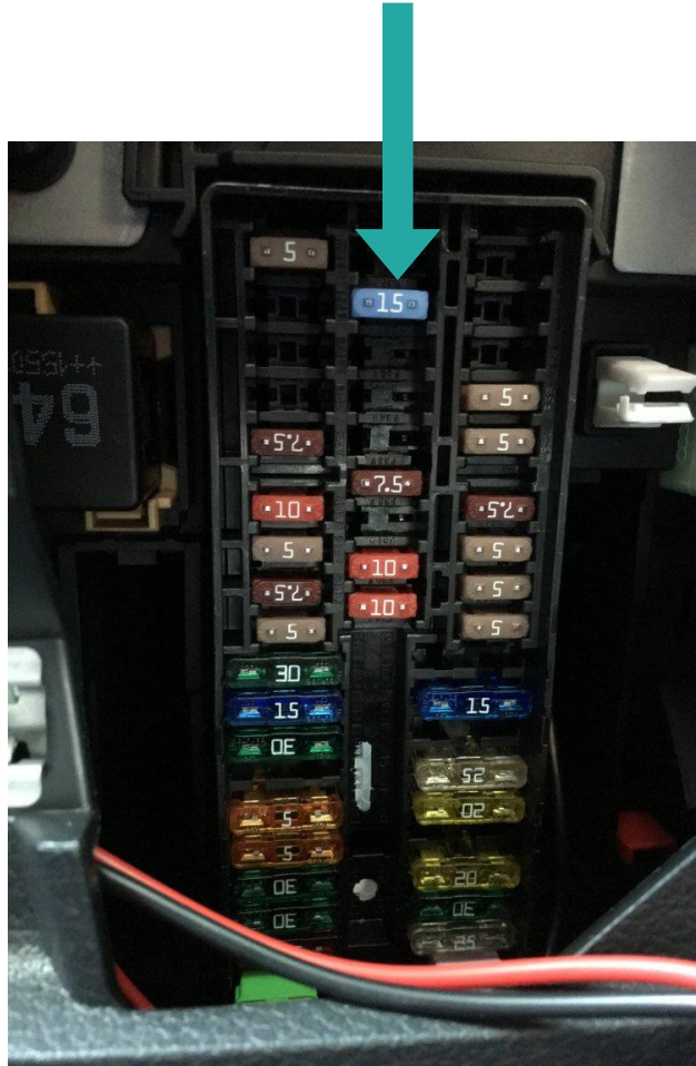
Remove the 15amp fuse from the centre column second down
