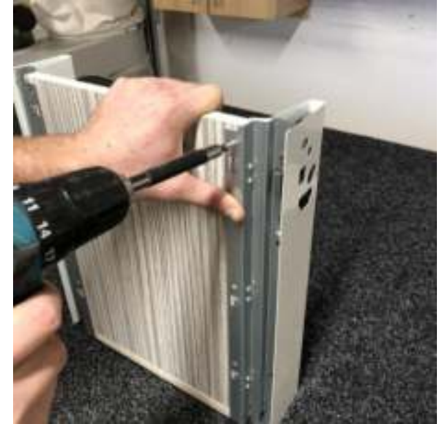
Fit the drawer base A5 using 15 mm screws, ensure the base is flush to avoid gaps
