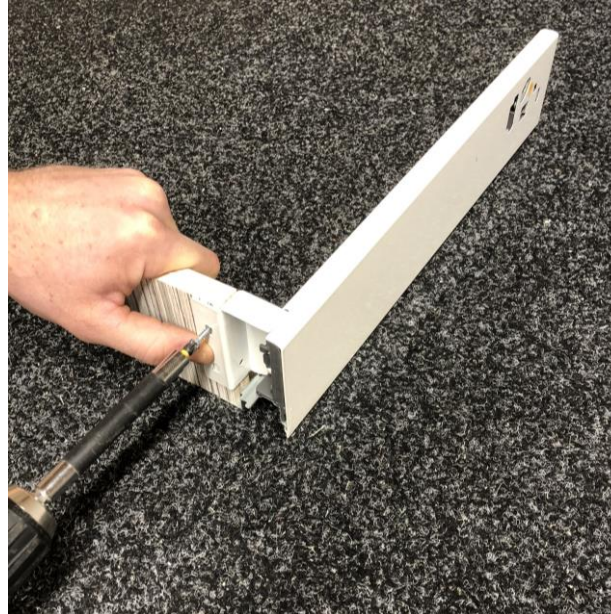
Fit the drawer rear using 16mm screws
