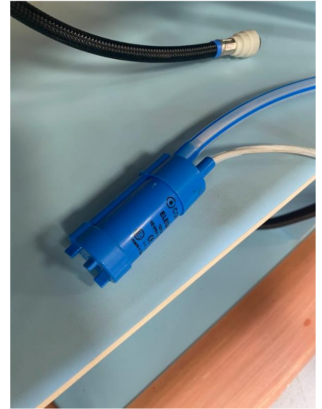
Fit the pipe to the water pump
