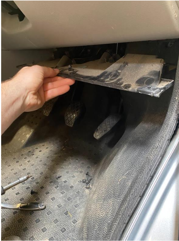
Remove the lower panel on the drivers side
