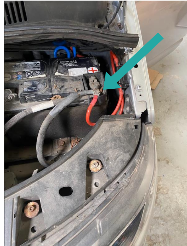
Connect the red split charge cable stud to the vehicle battery live
