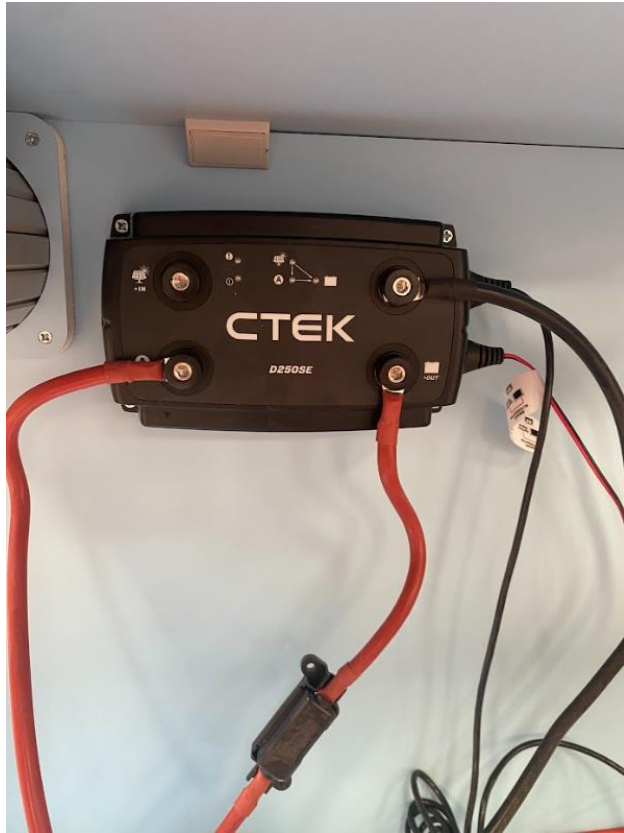
Screw the CTEK split charge into position, you will require 25mm screws
