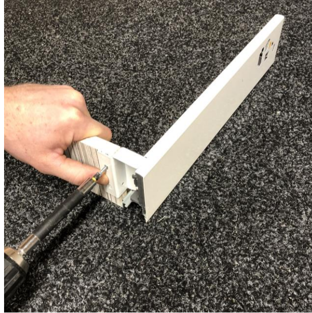
Fit the drawer rear using 16mm screws
