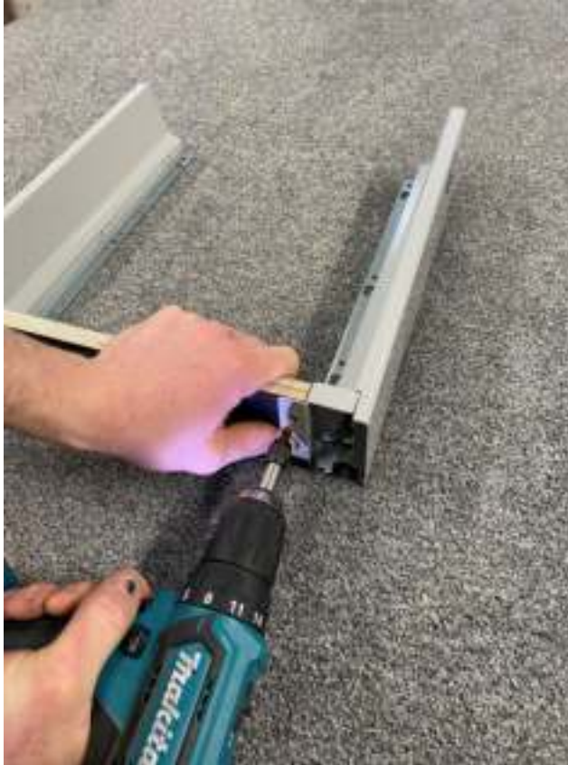
Fit the drawer rear using 15mm screws.
