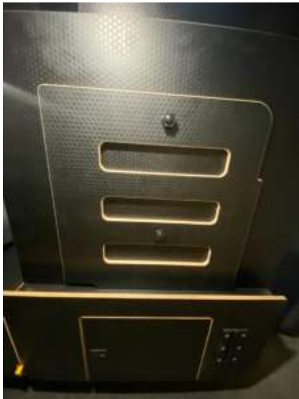
Test fit F1 in the transit position using the M6 hand wheels
