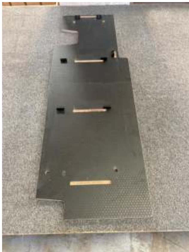
Prepare the floor C4 with blocks ready to assemble
