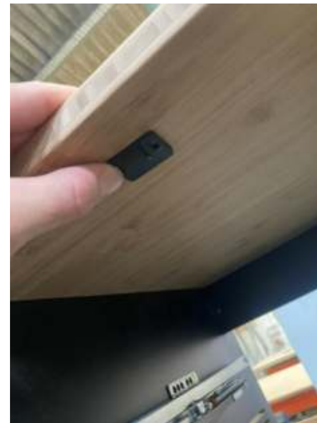
Fit the strike plates for the drawer and C13 door
