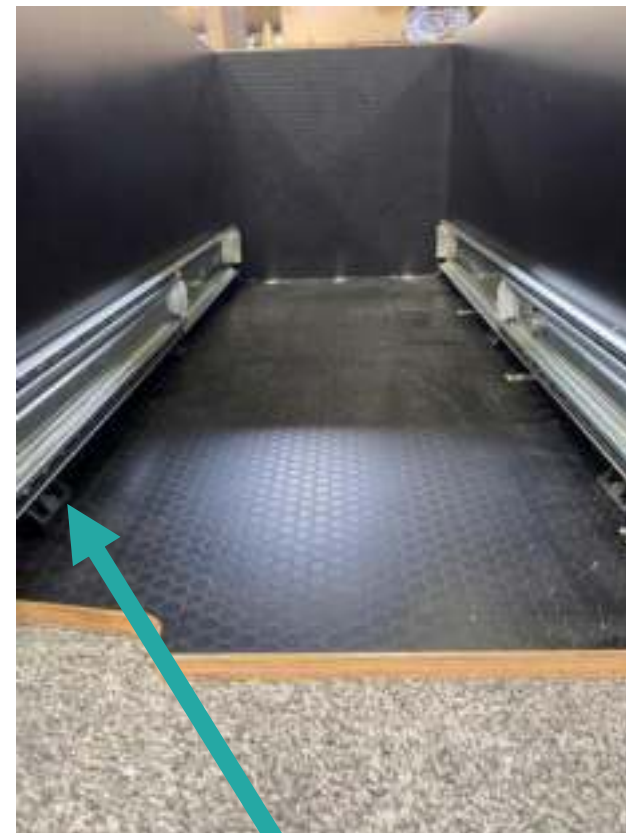
Continue to the rear, 4 either side is suffice, use a drill extension to access (remove and runners if necessary)
