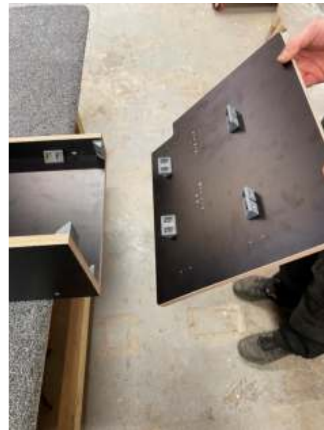
Fit A10 as per picture using pilot holes to align
