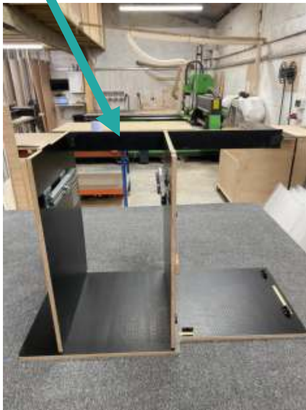
Fit the rear support C4 with C1 and C2 into the floor base
