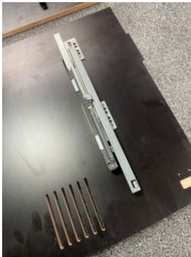
Fit the drawer runners to C1 and C2
