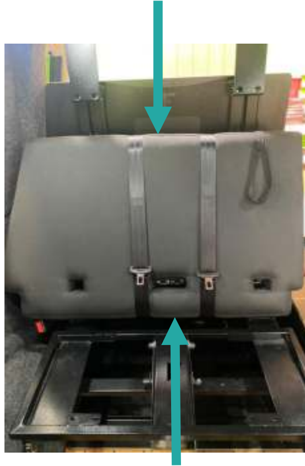
Offer the seat rear, the top and bottom will align with the framework
