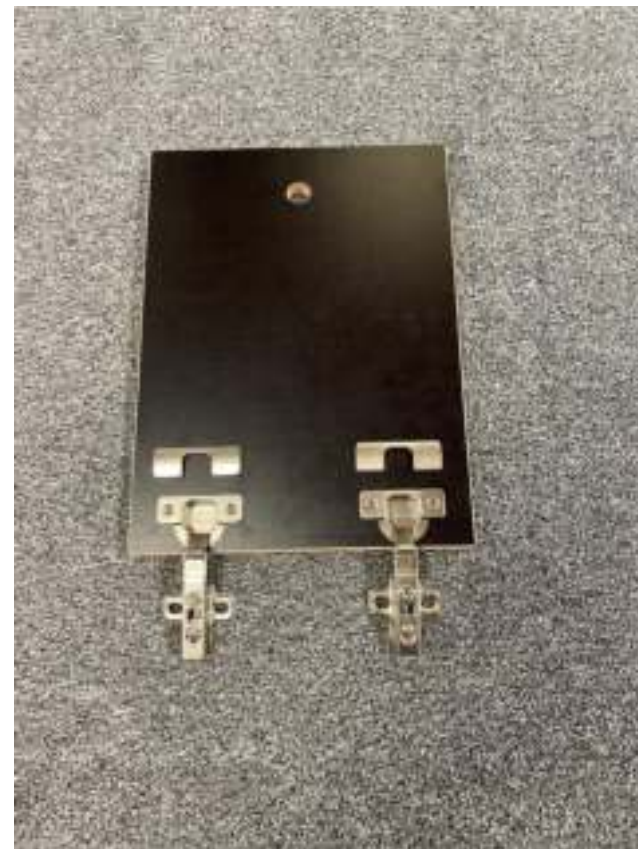
Fit overlay hinges to E11
