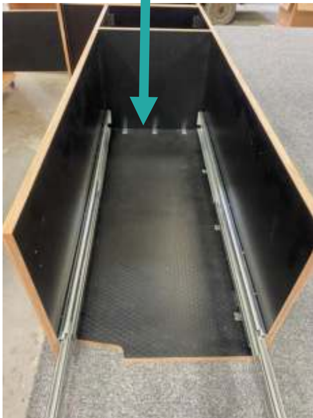
Slide A8 into place and fit with blocks
