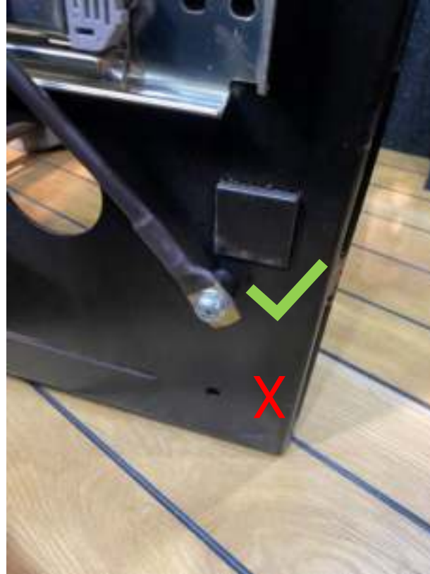
Fit the seat belt to the top mounting hole
