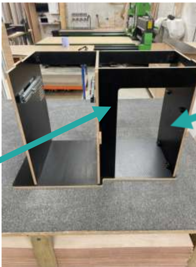
Fit the right end panel C3 and the face C5, unclip C5 door for easier fitting
