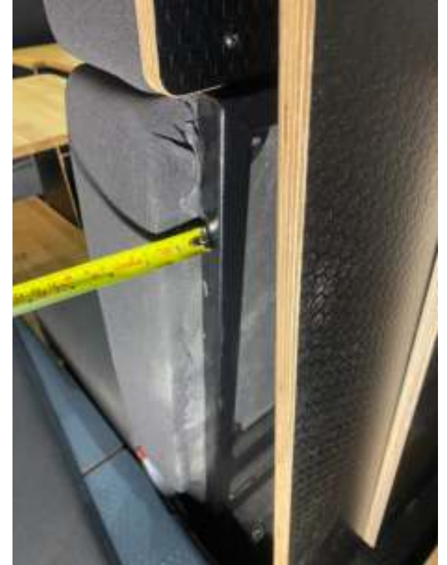
For correct lateral positioning, the seat rear should overhang the frame by 35mm
