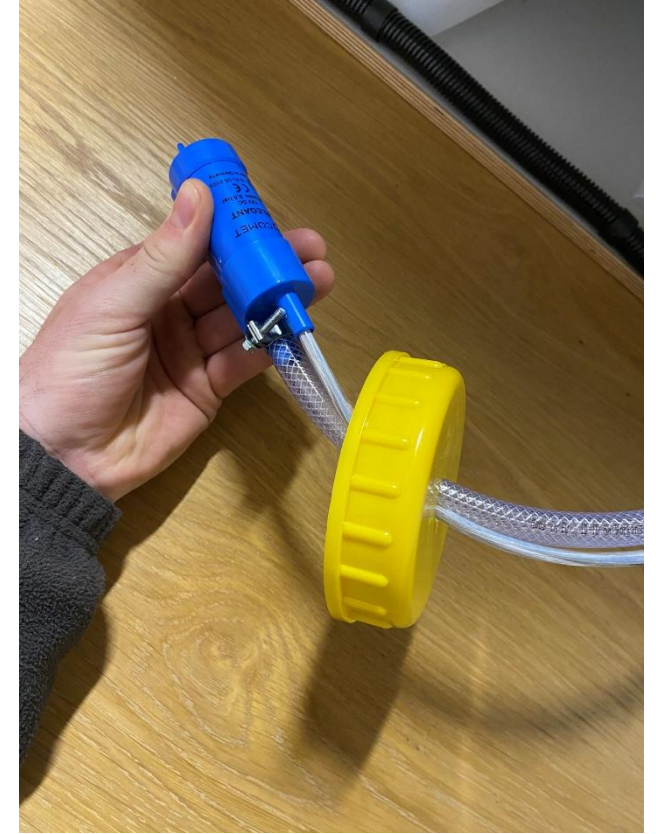
Attach the freshwater pipe to the pump with a jubilee clip, then feed through the yellow lid hole along with pump cable
