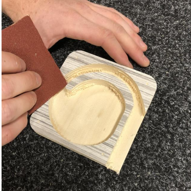
Sand the internal wheel to allow the tambour to glide
