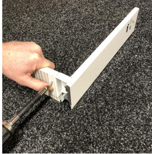
Fit the drawer rear using 16mm screws
