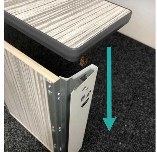
Clip the face into the side runners, if you have the deeper drawer attach the bar also
