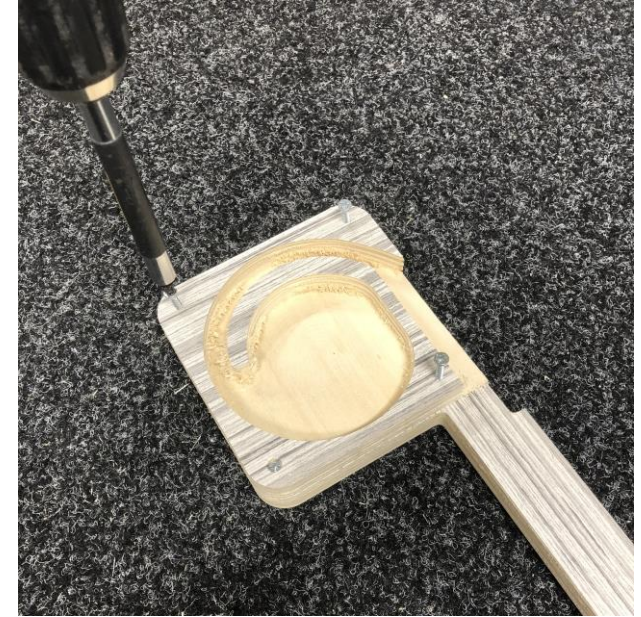
Screw the wheel to the support ensuring it sits flush all round using 25mm screws
