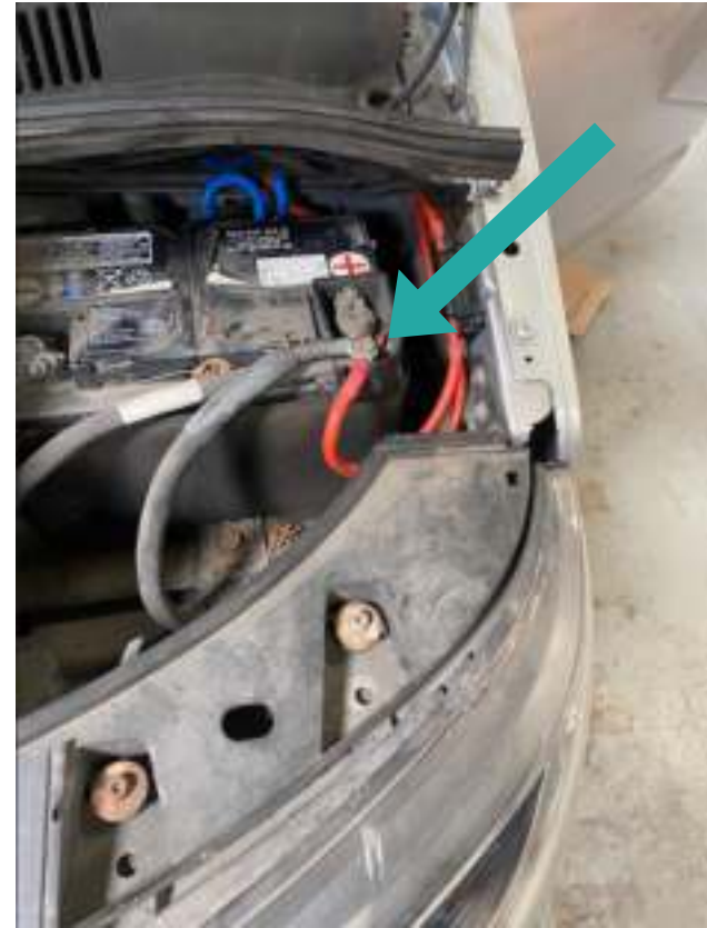
Connect the red split charge cable stud to the vehicle battery live
