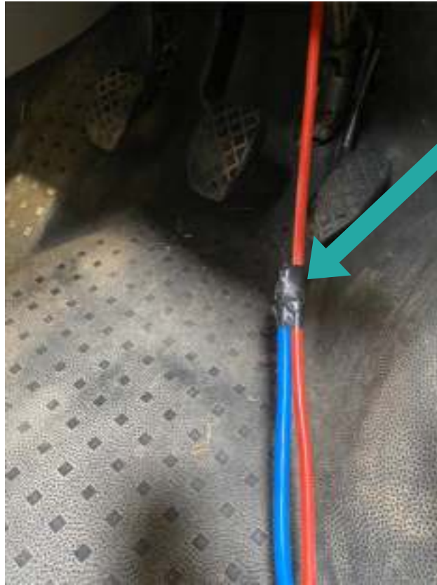
Tape the end of the blue approximately 2m from the red end
