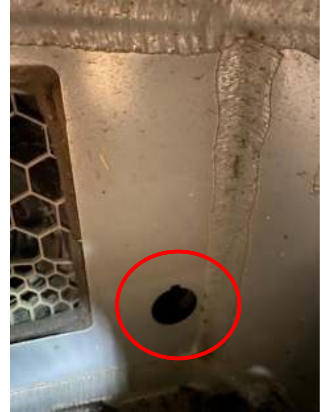
Fit a 25mm rubber grommet
