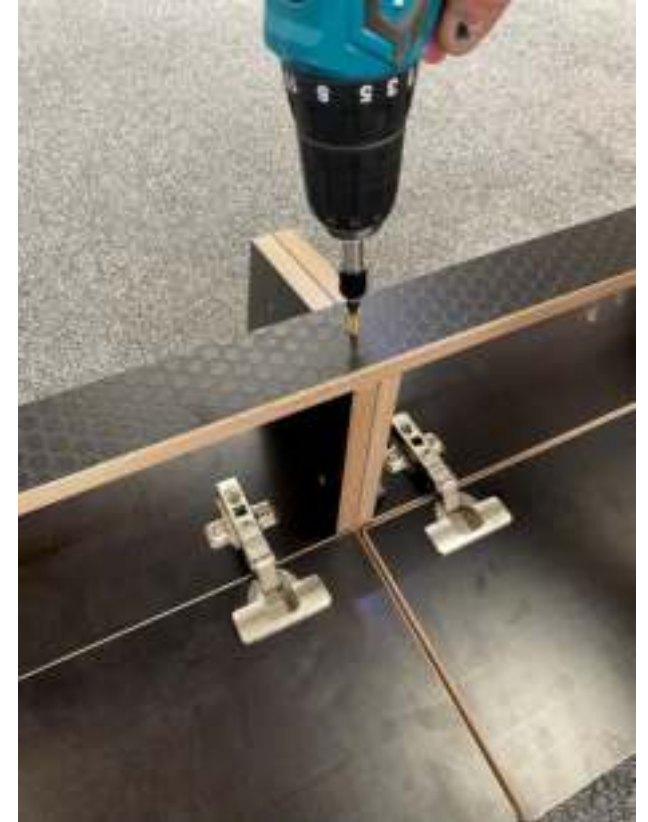
Fit D6 using the blocks to D4 and D5 and a 25mm screw into the centre dividers as per picture
