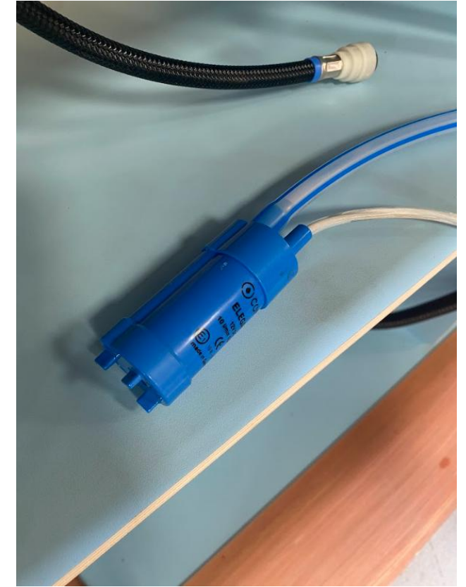
Fit the pipe to the water pump
