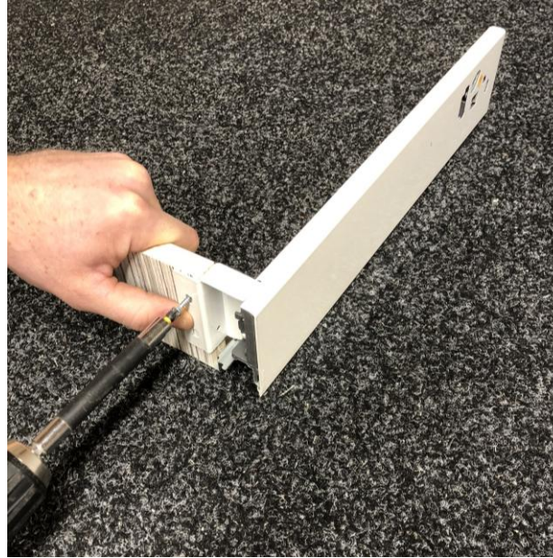
Fit the drawer rear using 15mm screws
