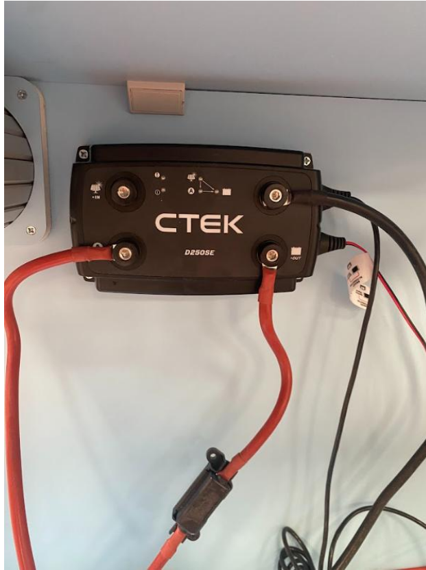
Screw the CTEK split charge into position
