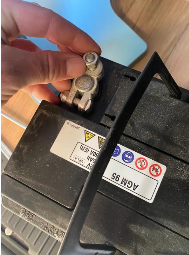
Attach the battery terminals
