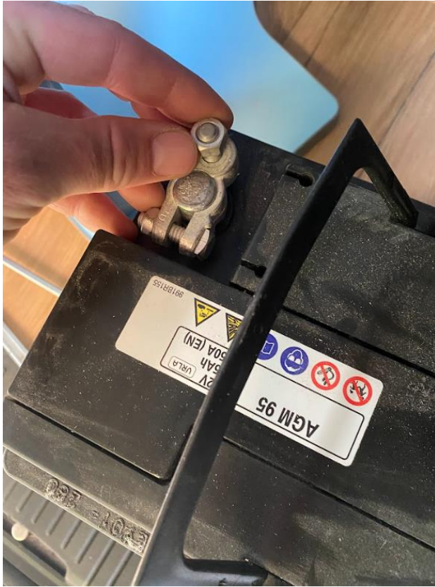
Attach the battery terminals
