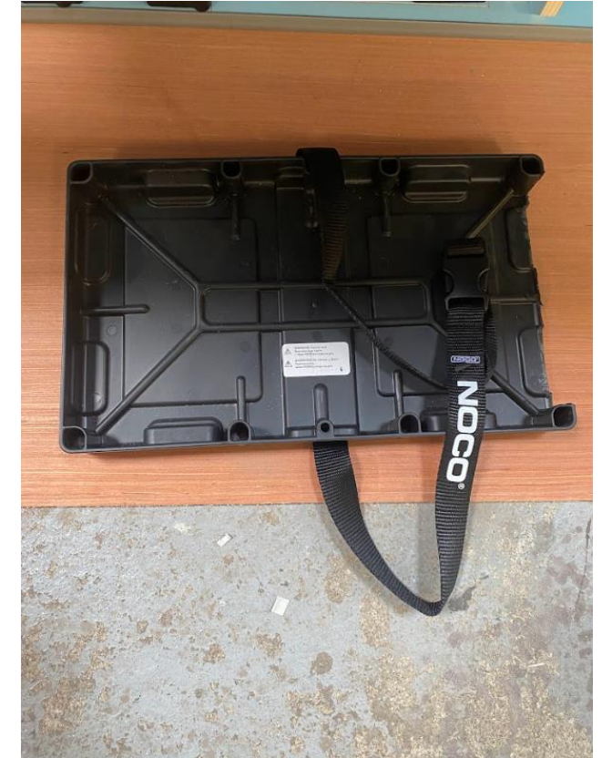
Before fitting the battery tray remember to feed the strap underneath
