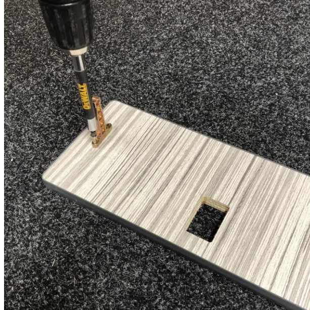
Screw the drawer face mounts into the pilot holes with the 4 x large head screws provided with the drawer box
