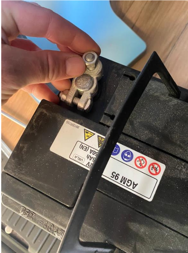
Attach the battery terminals
