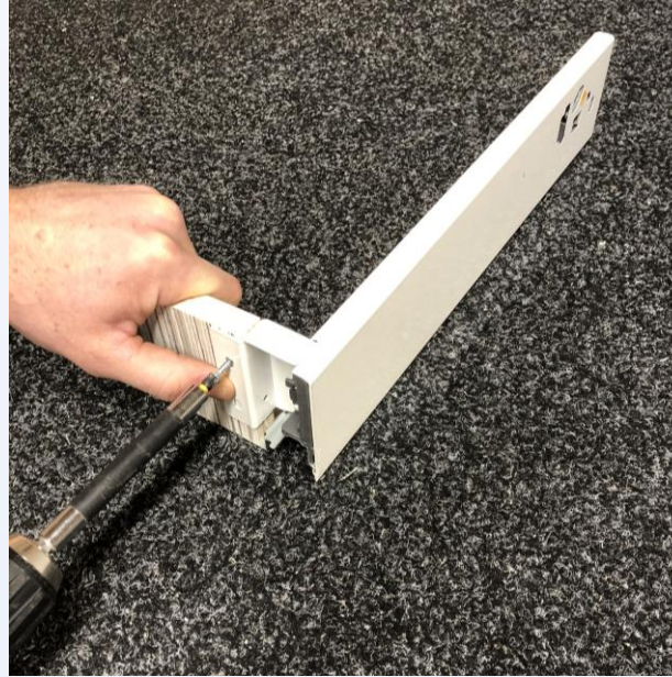
Fit the drawer rear using 16mm screws
