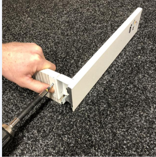
Fit the drawer rear using 16mm screws
