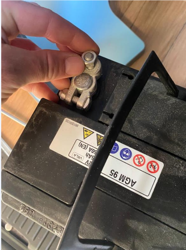
Attach the battery terminals
