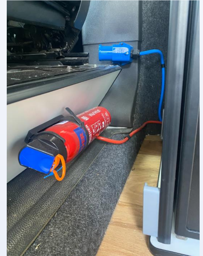
Reattach the battery cover and p-clip cables neatly
