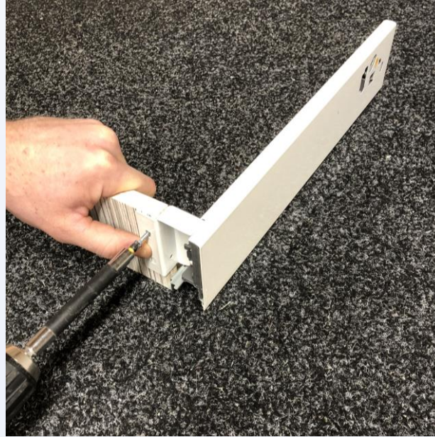
Fit the drawer rear using 16mm screws
