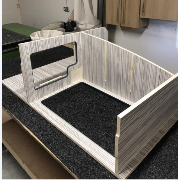
Slot the bottom shelf, divider and lid shelf into the rebates DO NOT SCREW
