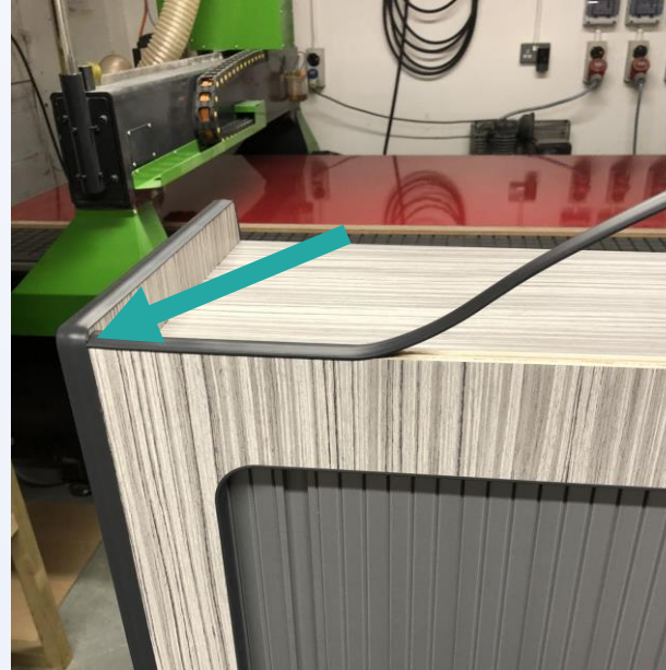
T Trim the Wardrobe face starting on the arrow. Trim lip outside
