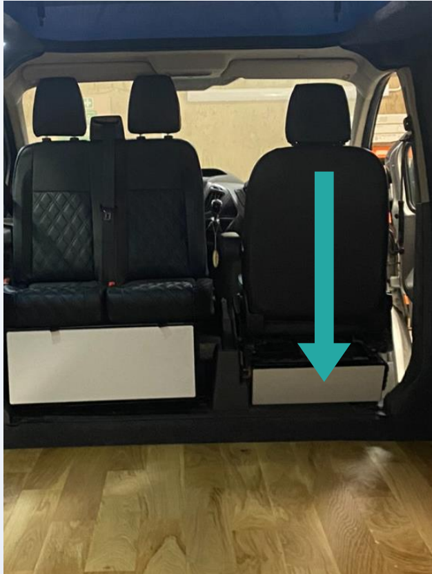
Locate and access the vehicle battery beneath the driver's seat
