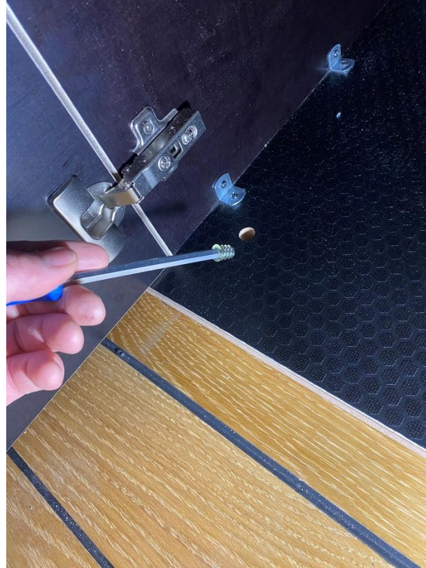
Screw a 6mm threaded insert into the hole in the van floor
